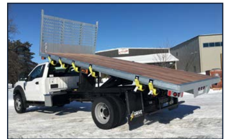
GALVANIZED STEEL WITH WOOD FLOOR
