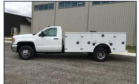
Voth's all aluminum service body is manufactured in rugged, corrosion-resistant 5052-H32 marine grade aluminum. Heavy gauge construction provides additional strength, reducing maintenance and maintaining improved fuel efficiency and payload capacity at 45% lighter than steel.
