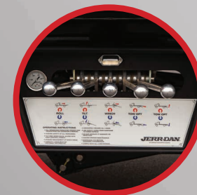
DUAL LIGHTED CONTROL STATIONS
