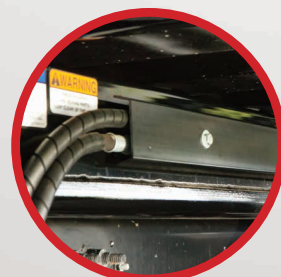
HYDRAULIC STEEL LINES WITH PROTECTIVE COVER
